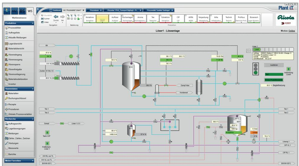
Plant iT process picture of the sugar dissolver
