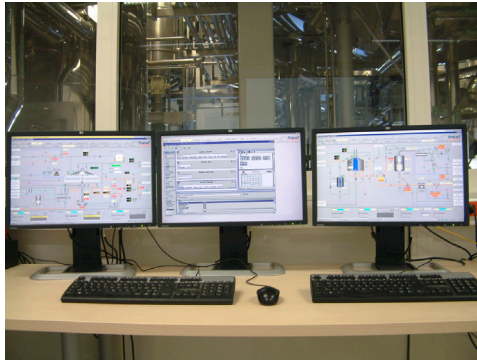
The brewmaxx materials management combined with the Report Designer provides the basis for reporting with batch tracking, material balances and loss determination.
